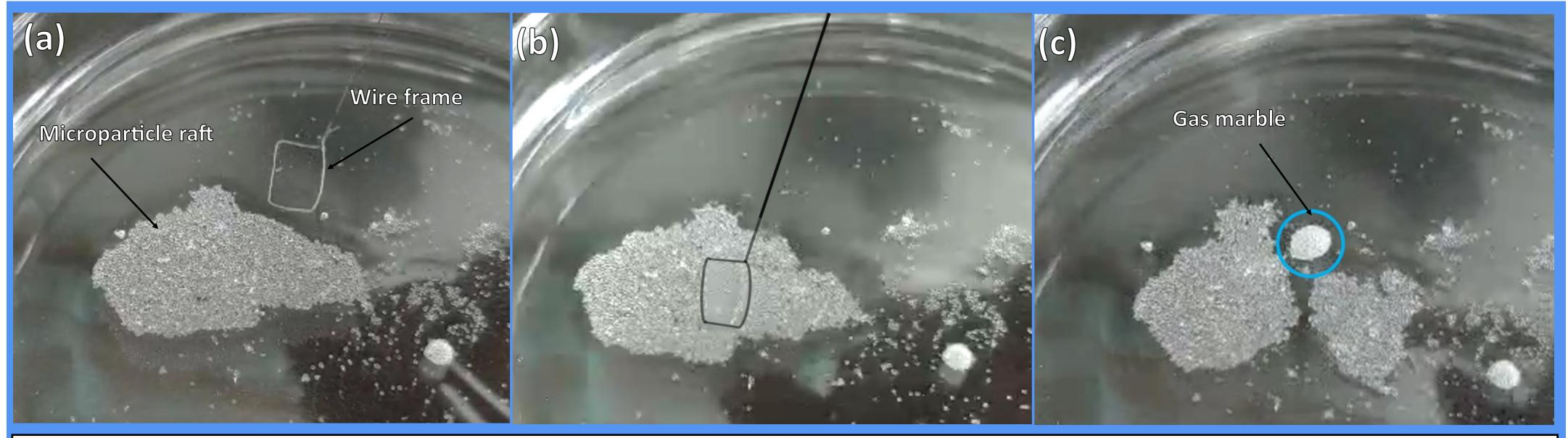
Figure 4. Process of gas marble production. In (a), the particle raft and wire frame can be seen. In (b), the wire frame is submerged under the raft (frame drawn on for clarity). In (c), the wire frame has been pulled upwards and a gas marble has formed.
